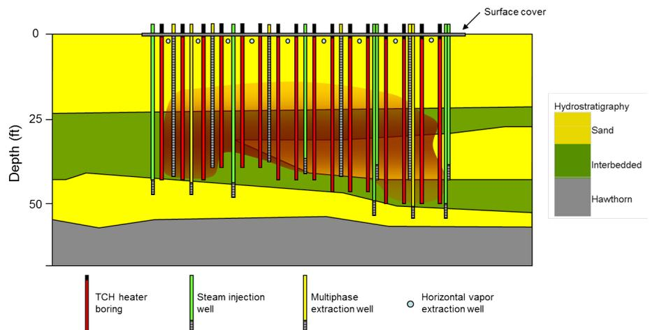
Vapors were extracted from the subsurface under vacuum and treated through a thermal oxidizer/acid gas scrubbing prior to discharge to the environment. Water was extracted and treated through various synthetic medias to target chlorinated Volatile Organic Compounds (VOCs) as well as 1,4-dioxane.
