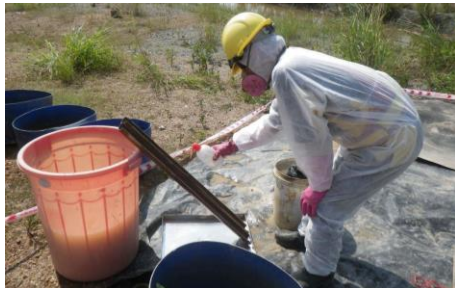
Decontaminating sampling equipment (Photo: CDM Smith)
