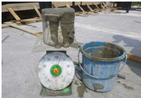
Concrete testing (Photo: CDM Smith)
